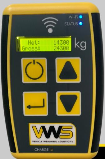
Once connected the wireless handheld will show the current Net and Gross Weight.
